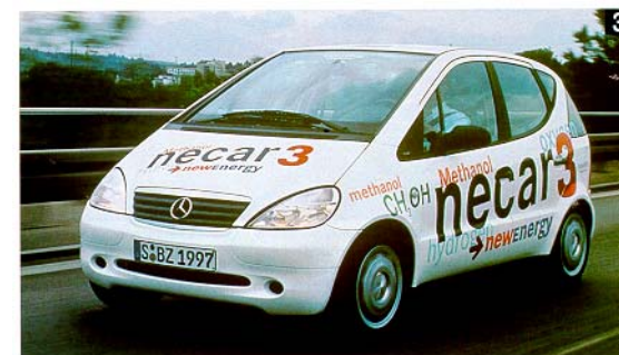
Necar 3 is powered by 50kW of fuel cells, which are supplied with hydrogen from an on-board methanol reformer
