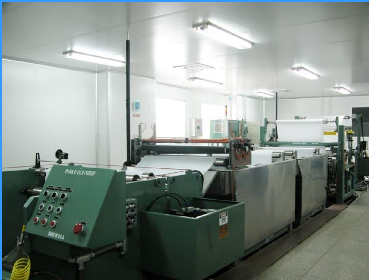
Fig.2-5 RO membrane production line with a capacity of 1.2 \times 10^6 \text{m}^2/\text{a}
