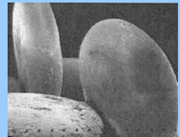
NaCl crystals grown in a rotating flow
